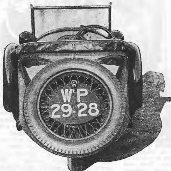
*Morgans are now fitted with spare wheels and on the sports two-seater the tail is specially shaped to accommodate this desirable fitting.*
