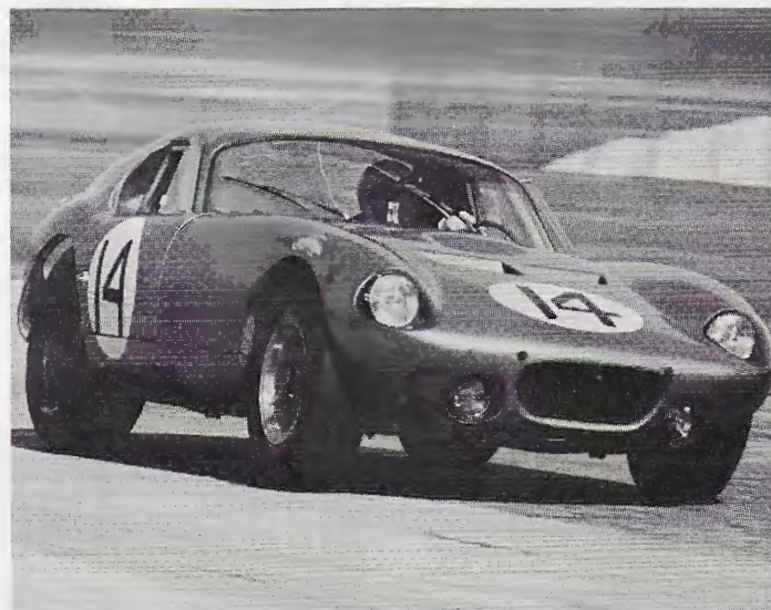
Bob Holbert and the Shelby American Cobra coupe just before that fateful pit stop at Daytona. Changes made in the coupe Holbert drove at Sebring included, according to Carroll Shelby: "A couple of oil pumps, air to the front brakes, and 15 more hp."
